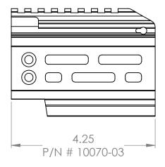
MAXIMUM SUPRESSOR DIAMETER SHOULD NOT EXCEED 1.57". TO MOCKUP AND ANTICIPATE OUR HANDGUARDS ABILITY TO SHROUD SUPPRESSORS, USE A STRAIGHT RULE OR TAPE TO MEASURE FROM THE FRONT SURFACE OF YOUR UPPER RECEIVER FORWARD AS NOTED ON THIS PAGE. DIMENSIONS SHOWN ARE ACTUAL AND TRUE TO FORM.
